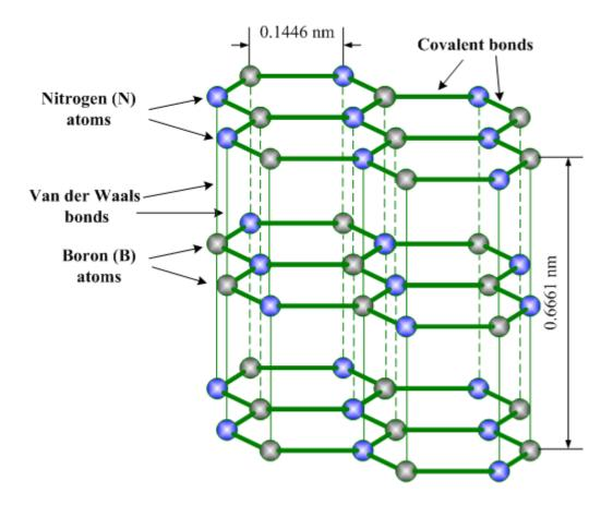
The layered structure allows sliding movement of the parallel planes. Weak bonding between the planes provides low shear strength in the direction of the sliding movement but high compression strength in the direction perpendicular to the sliding movement.
